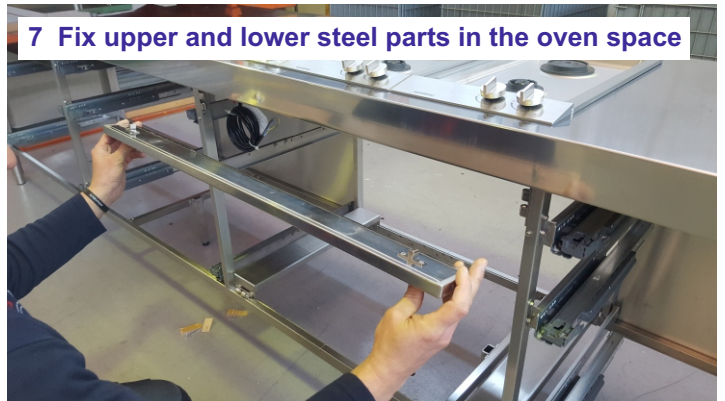
7 Fix upper and lower steel parts in the oven space
